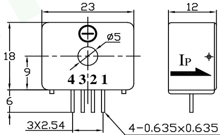
Elucidation: 1:+15V 2:0V(GND) 3:V<sub>OUT</sub> 4:-15V
